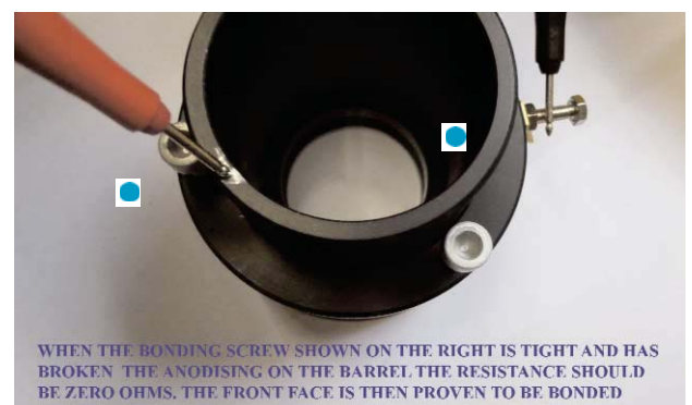
REMOVE A SMALL PART OF THE ANODISING FROM THE BARREL TO EXPOSE THE ALUMINIUM FOR TESTING THE BONDING CONNECTION
