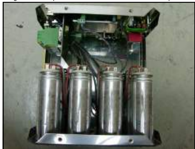
Fig. 6.11.3-2: Opened AC Control Box from Panda 30 upwards
