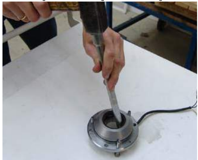
Fig. 7.12.2-8: Knocking out the ball bearing
