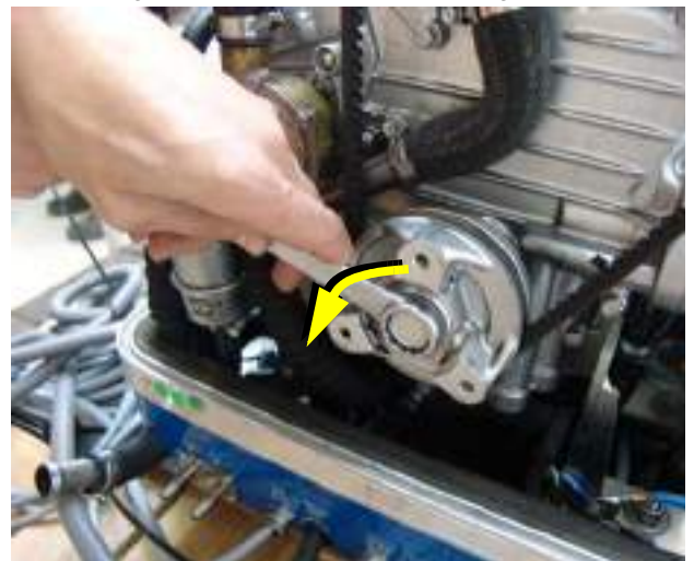
Fig. 7.10.1.3-8: Hold up the driving shaft
