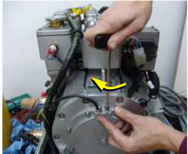
Fig. 7.12.2-34: Screw in the ventilation screw
