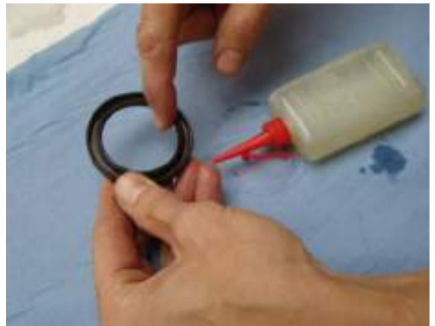
Fig. 7.12.2-14: Mounting the shaft sealing ring
