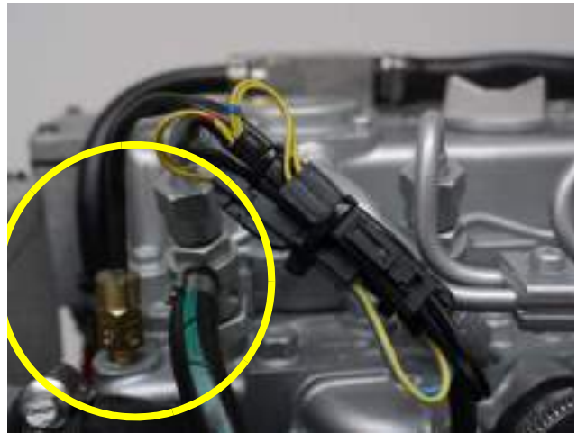
Fig. 4.3.4-1: Thermo-switch at cylinder head
