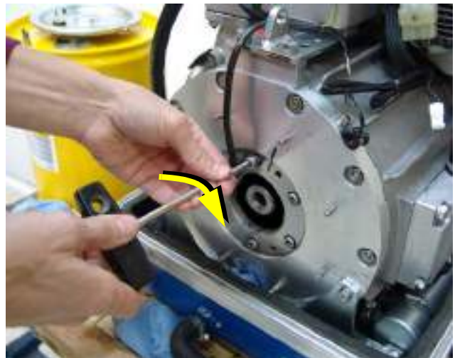
Fig. 7.12.2-25: Mount the thread rod
