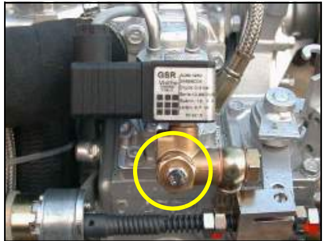
Fig. 7.13-2: Ventilation screw at the fuel solenoid valve
