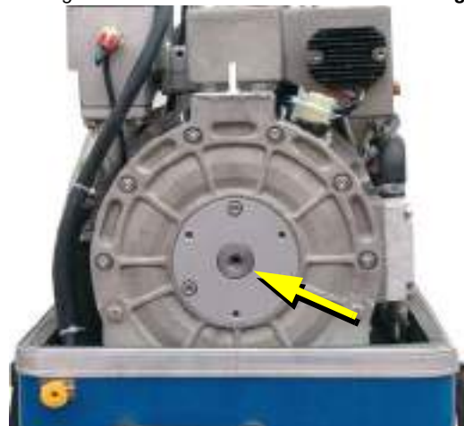
Fig. 7.10-1: Grease lubricated backend bearing
