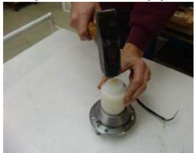
Fig. 7.12.2-10: Dismount the shaft sealing ring
