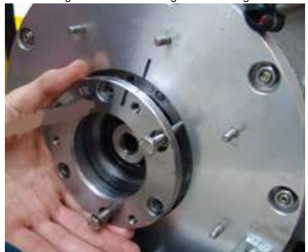
Fig. 7.10.1.3-2: Bearing case mounting
