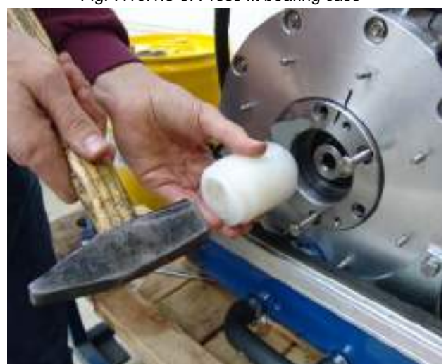
Fig. 7.10.1.3-3: Press fit bearing case
