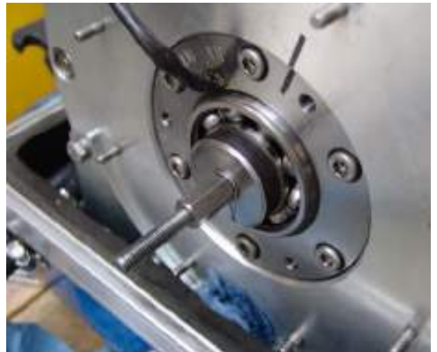
Fig. 7.12.2-27: Mounting the ball bearing
