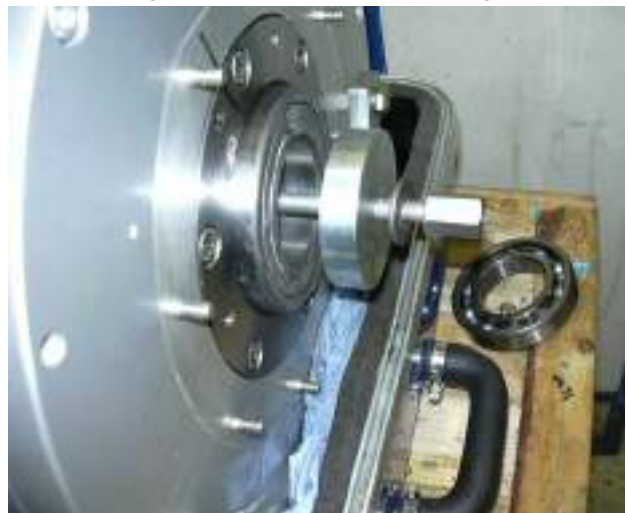
Fig. 7.10.1.3-6: Put on ball bearing
