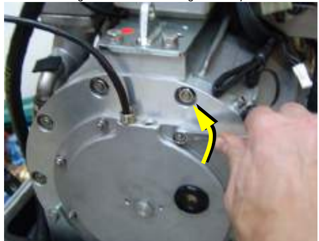
Fig. 7.12.2-3: Demounting the oil cap
