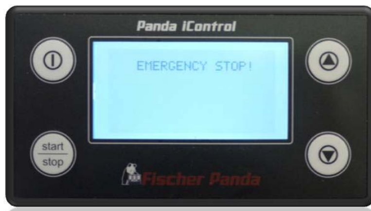
Fig. 13.5-2: Panel shows Emergency Stop
