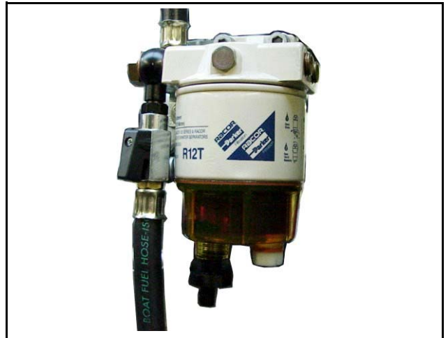
Fig. 8.11-1: Pre-filter with water separator
