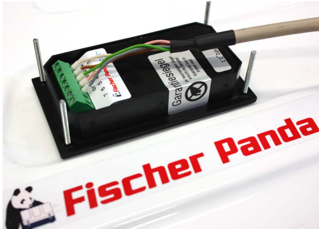
Fig. 14.2.1-1: Panda iControl2 panel with panel connecting cable and closed housing
