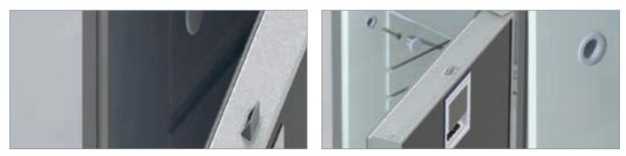
The cabinet can be directly installed from the interior of the fridge thanks to the easy fix installation system. The external flange is no longer needed for the installation. An innovative internal bushing structure prevents the crushing of the insulated side wall.
