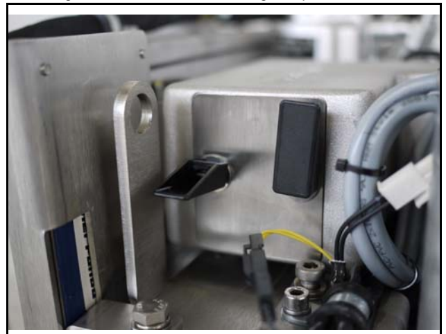
Fig. 7.10.2-3: Air suction housing with pull out holder
