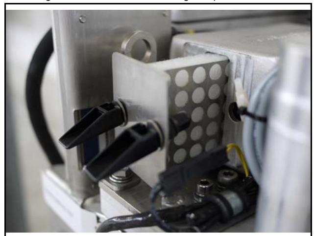
Fig. 7.10.2-3: Air suction housing with pull out holder
