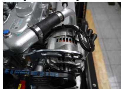
Fig. 7.10-3: Replacing the V-belt
