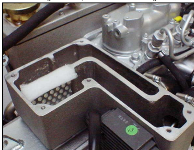
Fig. 7.11-2: Opened air suction housing
