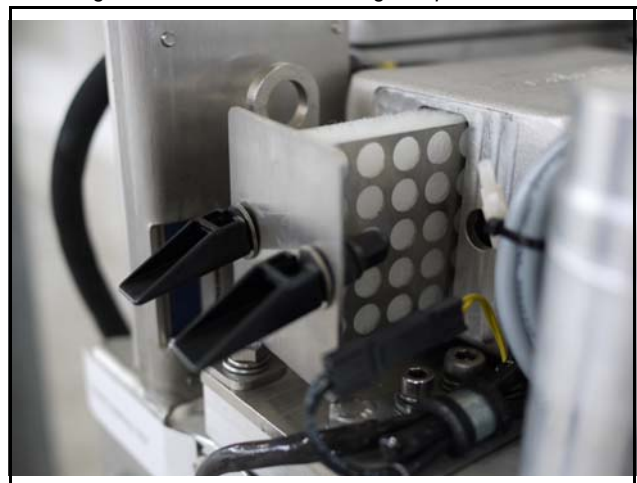
Fig. 7.11.2-3: Air suction housing with pull out holder
