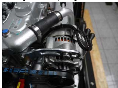
Fig. 7.11-3: Replacing the V-belt
