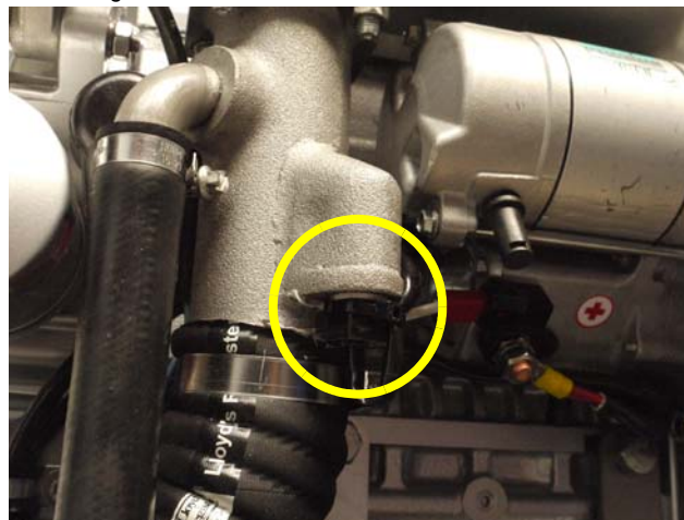
Fig. 4.3.6-2: Thermo-sensor at exhaust connection
