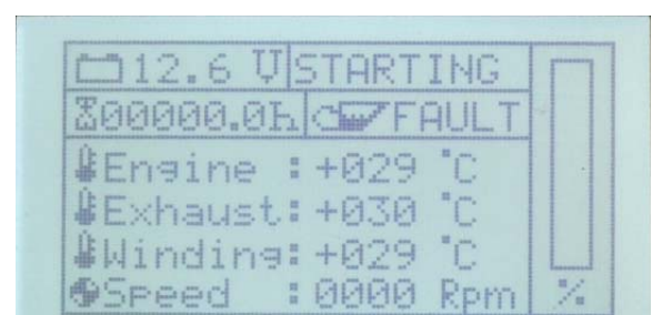
Fig. 12.3.3.2-2: Default display screen during start-up
