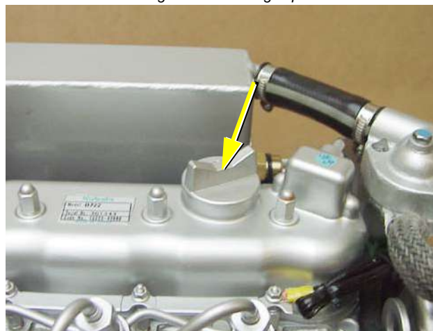
Fig. 7.8-2: Oil drain hose
