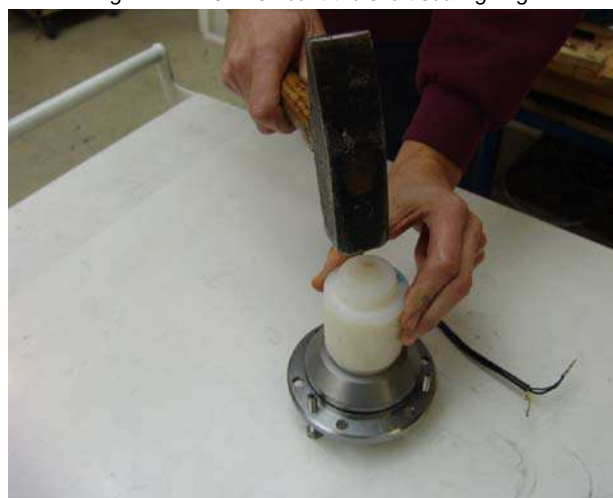
Fig. 7.12.2-10: Dismount the shaft sealing ring
