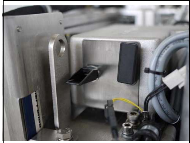
Fig. 7.14.2-2: Air suction housing with pull out holder
