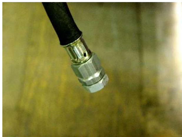
Fig. 7.8-2: Oil drain hose
