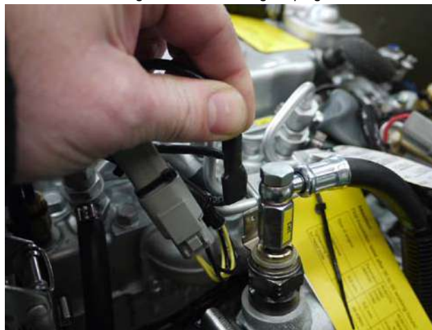
Fig. 7.21.1-2: Flame glow plug
