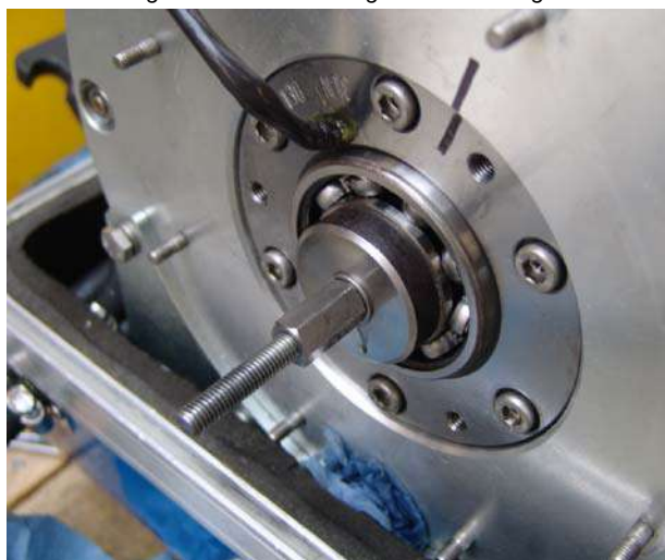
Fig. 7.12.2-27: Mounting the ball bearing
