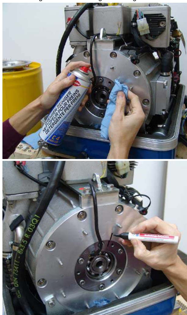
Fig. 7.10.1.2-1: Marking the bearing cover.
