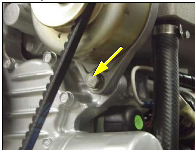
Fig. 7.14-2: Screw underneath the alternator
