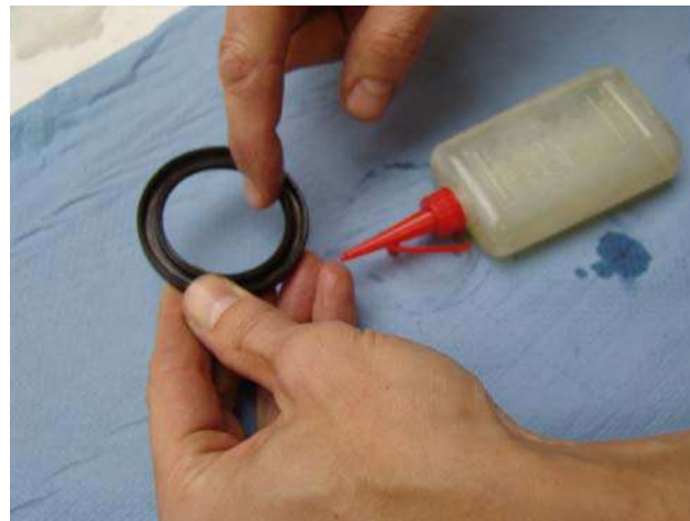
Fig. 7.12.2-14: Mounting the shaft sealing ring
