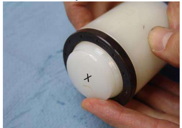
Fig. 7.12.2-17: Fitting the shaft sealing ring
