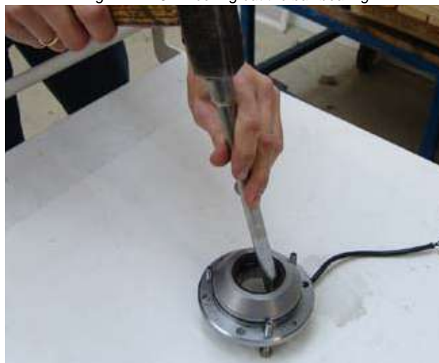
Fig. 7.12.2-8: Knocking out the ball bearing
