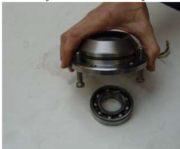
Fig. 7.12.2-10: Dismount the shaft sealing ring
