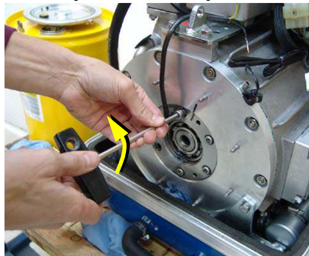
Fig. 7.12.2-5: Loosen fastening screws
