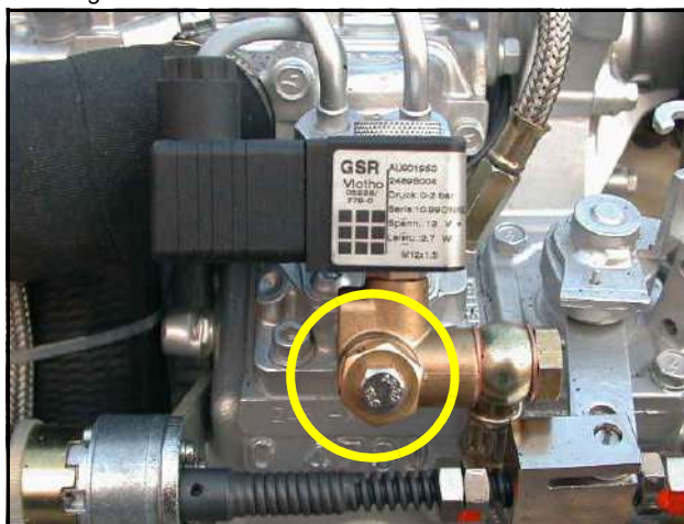
Fig. 7.13-2: Ventilation screw at the fuel solenoid valve
