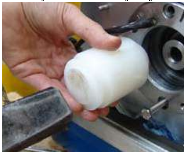
Fig. 7.12.2-23: Mount the bearing housing
