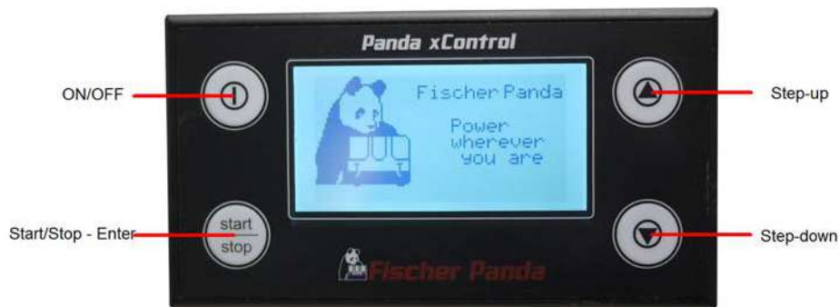
Fig. 4.3.1-2: xControl CP-G Reverse Sidel
