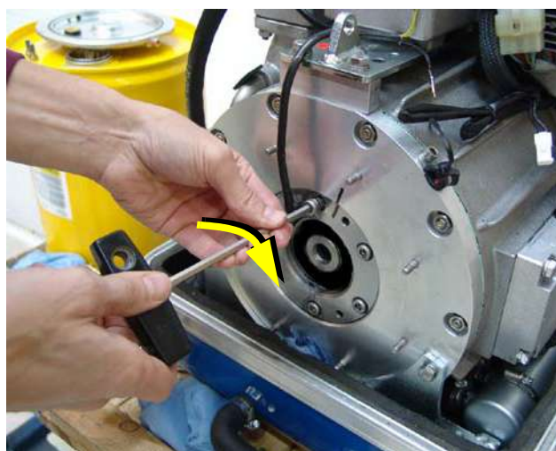
Fig. 7.12.2-24: Tighten the fastening screws
