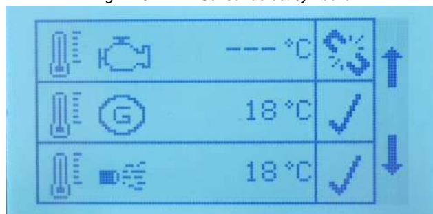
Fig. 11.6.1.1-1: Sensor defect symbolic
