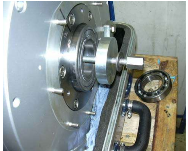
Fig. 7.10.1.3-6: Put on ball bearing
