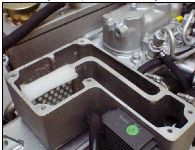
Fig. 7.14-2: Opened air suction housing
