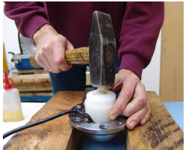
Fig. 7.12.2-17: Fitting the shaft sealing ring
