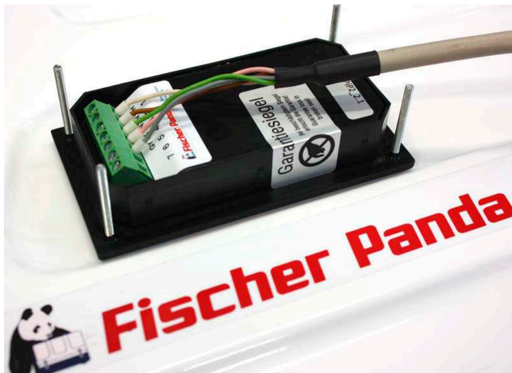
Fig. 16.2.1-1: Panda iControl2 panel with panel connecting cable and closed housing
