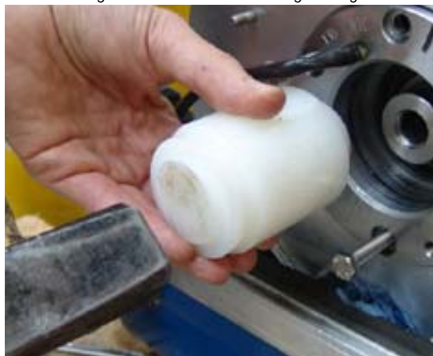
Fig. 7.12.2-23: Mount the bearing housing
