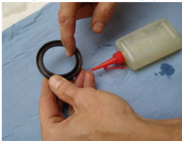
Fig. 7.12.2-14: Mounting the shaft sealing ring
