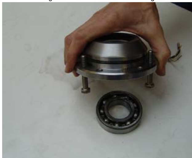
Fig. 7.12.2-10: Dismount the shaft sealing ring
