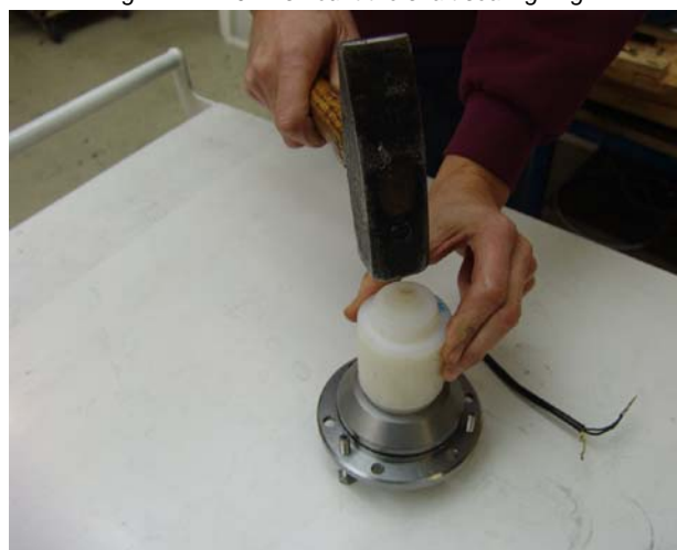
Fig. 7.12.2-10: Dismount the shaft sealing ring
