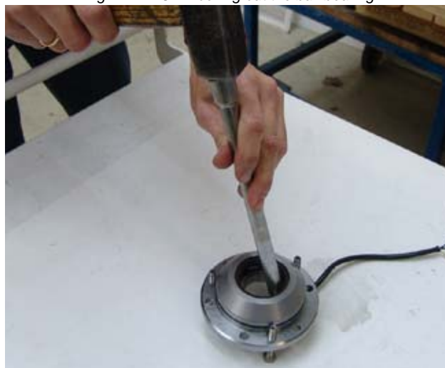
Fig. 7.12.2-8: Knocking out the ball bearing
