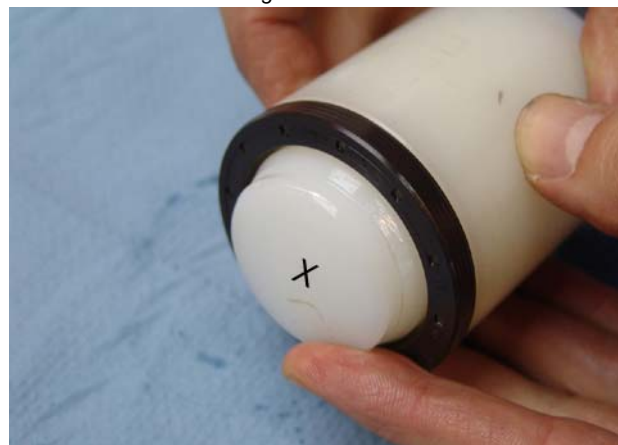
Fig. 7.12.2-17: Fitting the shaft sealing ring
