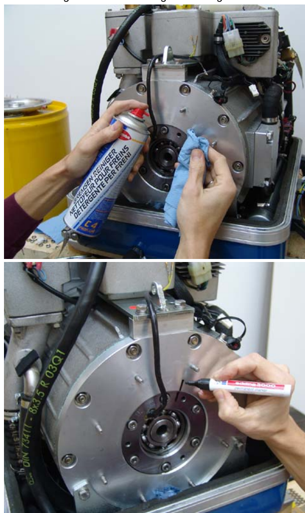
Fig. 7.10.1.2-1: Marking the bearing cover.
