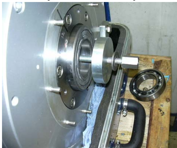
Fig. 7.10.1.3-6: Put on ball bearing
