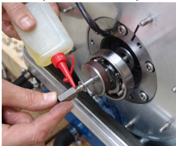
Fig. 7.12.2-26: Mount the ball bearing
