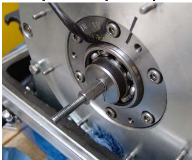
Fig. 7.12.2-27: Mounting the ball bearing
