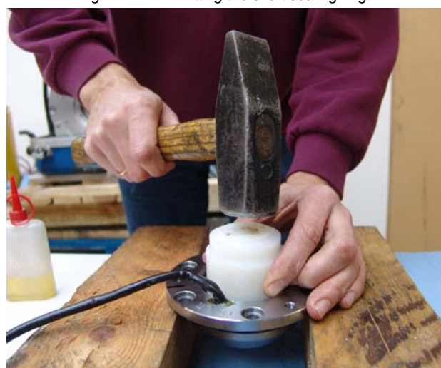
Fig. 7.12.2-17: Fitting the shaft sealing ring
