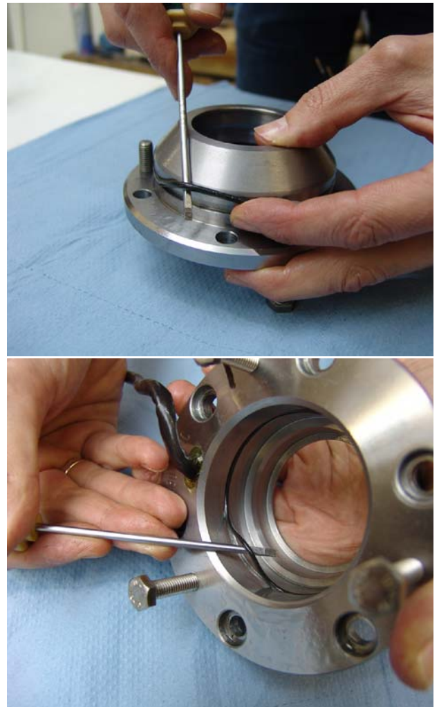
Fig. 7.12.2-12: Remove o-rings
