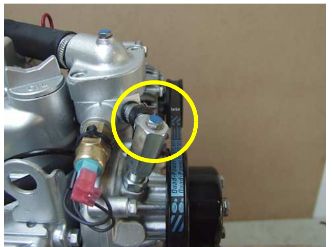
Fig. A.3.4-9: Ventilation screw cooling water pump
