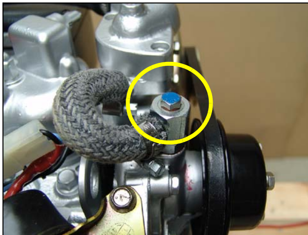
Fig. 5.3.3-8: Internal Cooling Water Pump
