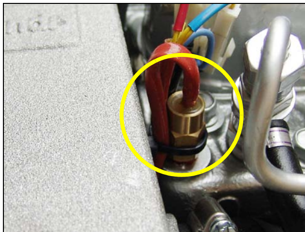
Fig. 5.3.7-1: Thermo-switch at Cylinder Head
