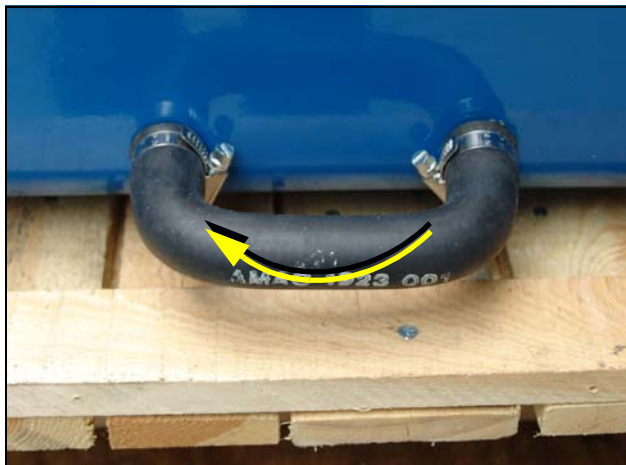
Fig. 5.3.2-4: Connection for Ventilation Valve
