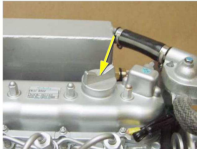
Fig. 6.4-2: Oil drain hose
