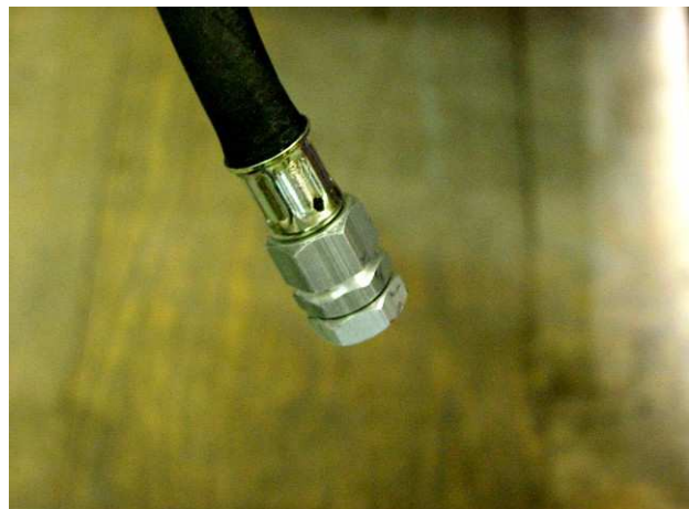
Fig. 6.4-2: Oil drain hose
