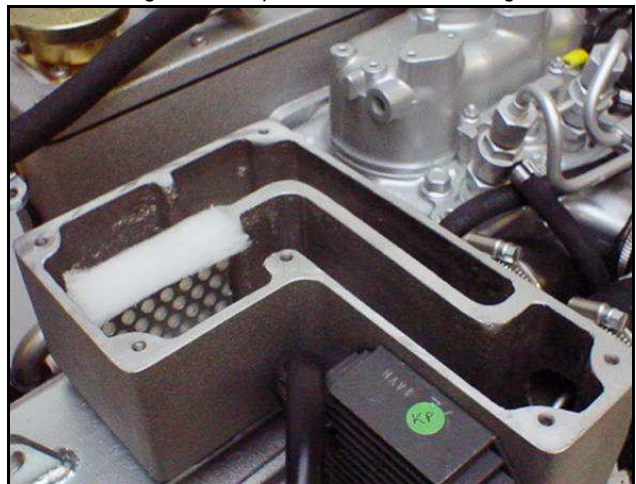
Fig. 6.6.3-2: Opened Air Suction Housing
