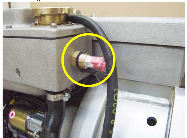
Fig. 4.3.7-2: Thermo-switch at exhaust elbow
