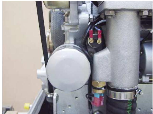
Fig. 4.3.8-4: Oil drain hose
