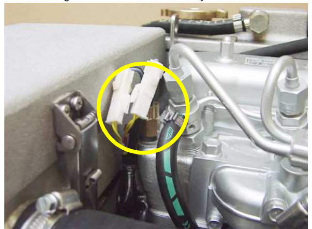
Fig. 4.3.7-1: Thermo-switch at cylinder head
