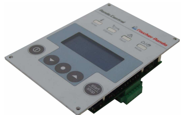
Fig. 4.2.7-3: Remote control panel
