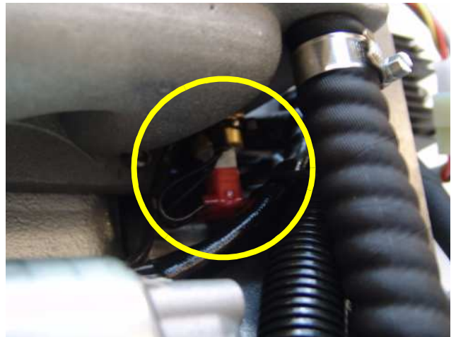
Fig. 4.2.5-2: Thermo-switch at exhaust elbow
