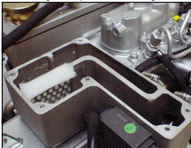
Fig. 7.11-2: Opened air suction housing
