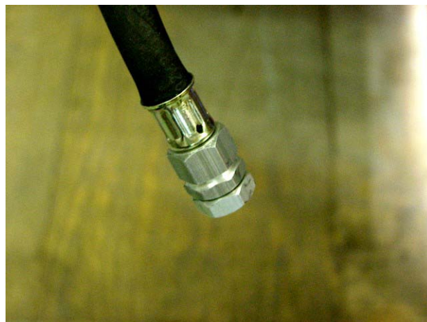
Fig. 7.8-2: Oil drain hose
