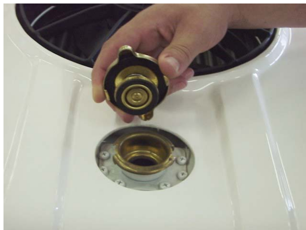
Fig. 7.6-5: Cooling water filler cap
