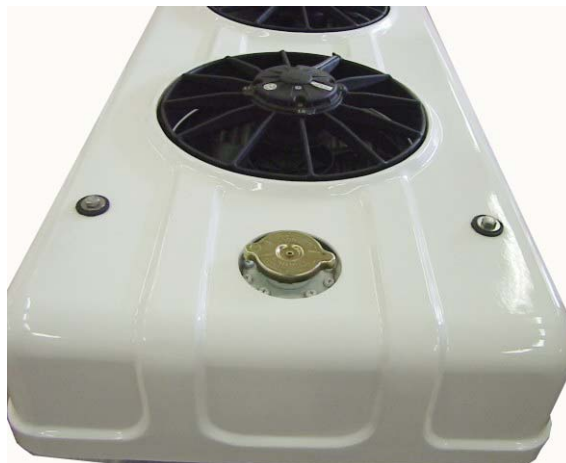
Fig. 7.6-4: Cooling water filler cap
