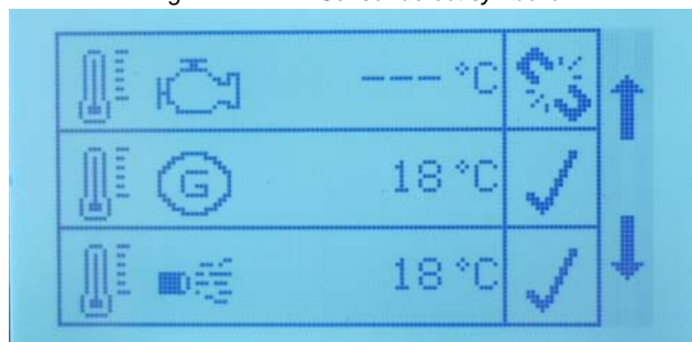
Fig. 11.2.1.1-1: Sensor defect symbolic
