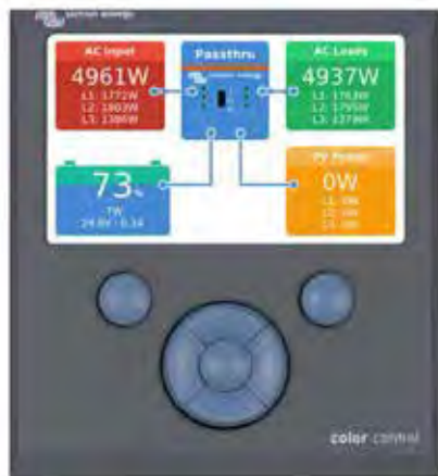
Color Control panel, showing a PV application
