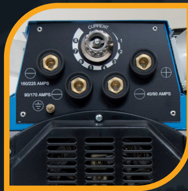
Welding Current Control
