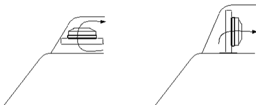
Figure 8: Two examples of top mount radiators
