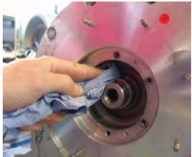
Fig. 9.12.2-19: Cleaning the shaft
