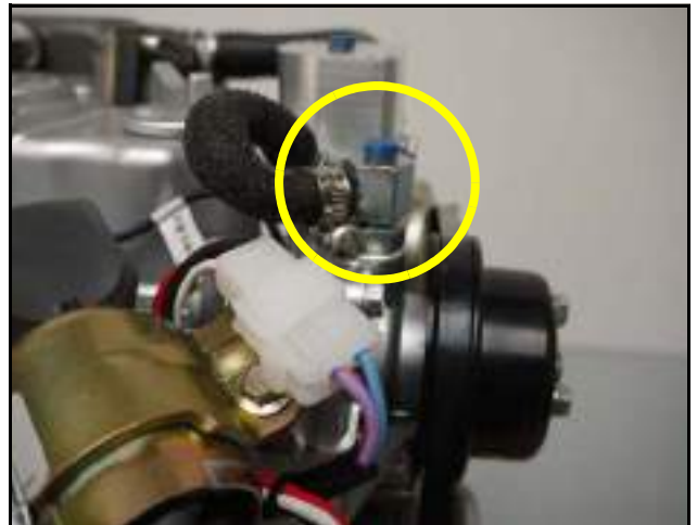
Fig. 6.3.2-8: Ventilation Screw Cooling Water Pump
