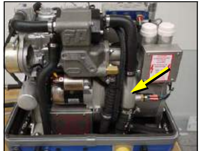
Fig. 6.3.1-5: Raw Water Injection
