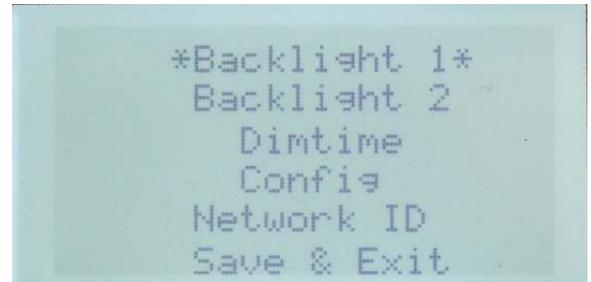
The Start/Stop button is used for confirming a selection in the set-up menu. If you confirm the row marked with the \* with the Start/Stop button, you will access the selected sub-menu.
