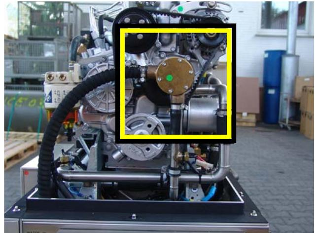
Remove the cover of the raw water pump by loosen the screws from the housing.
