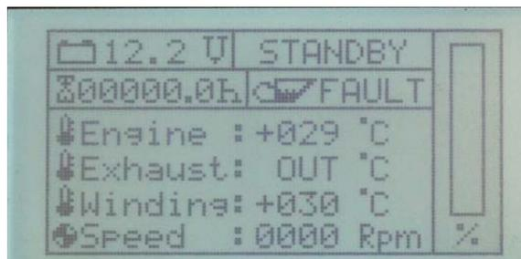
**Fault: „Winding“, winding temperature too high**
