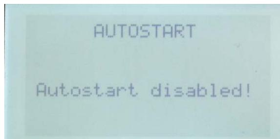
The activation/deactivation of the autostart function is then saved to the EEPROM of the control panel.
