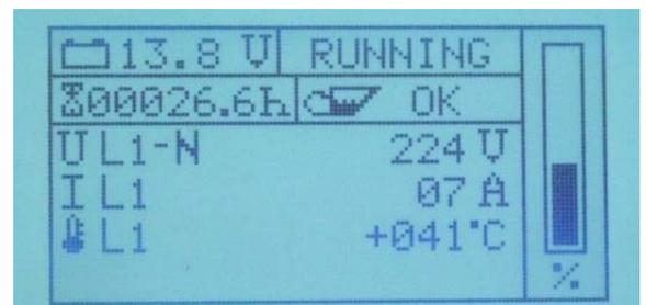
This screen provides the latest inverter output voltage of the single phases with the matching conductor current and the circuit board temperature. The inverter will be switched off at a circuit board temperature of 75 °C. You can access the inverter screen by actuating the cursor-up button while in operation mode.
