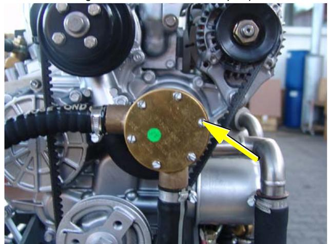
Fig. 7.13.1-4: Impeller pump
