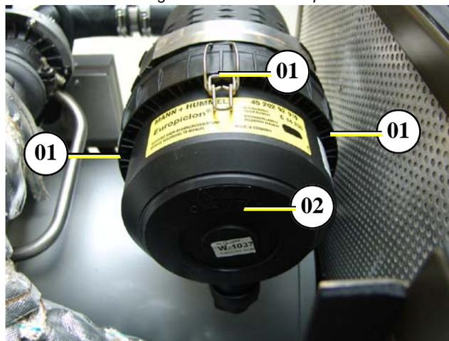
4. Remove the main element with a light turning movement completely from the inner support pipe.
