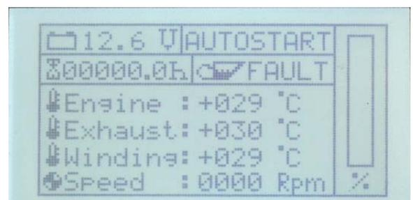
The autostart function will remain active even after the controller is switched off and on again with the On/Off button. To deactivate the autostart function, the flag in the EEPROM must be reset with "Disable". Siehe "Activating/deactivating the autostart function ("Autostart")" auf Seite 145.
