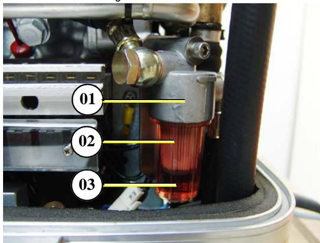
Unscrew the housing from its mount (left hand rotation).
