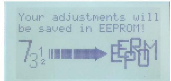
Then, the goodbye screen appears for 3 seconds, and the controller is switched off. At the next start of the controller, the changes will take effect.
