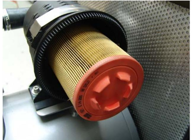
7. Blow out filter insert in folding direction maximum pressure: 5 bar.
