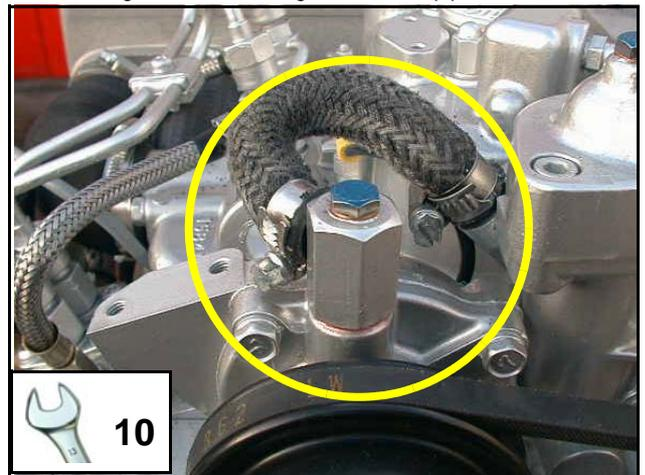
Fig. 7.11.1-2: Venting screw at the pipe socket
