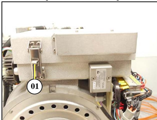
3. Open the air housing by pulling the cover.
