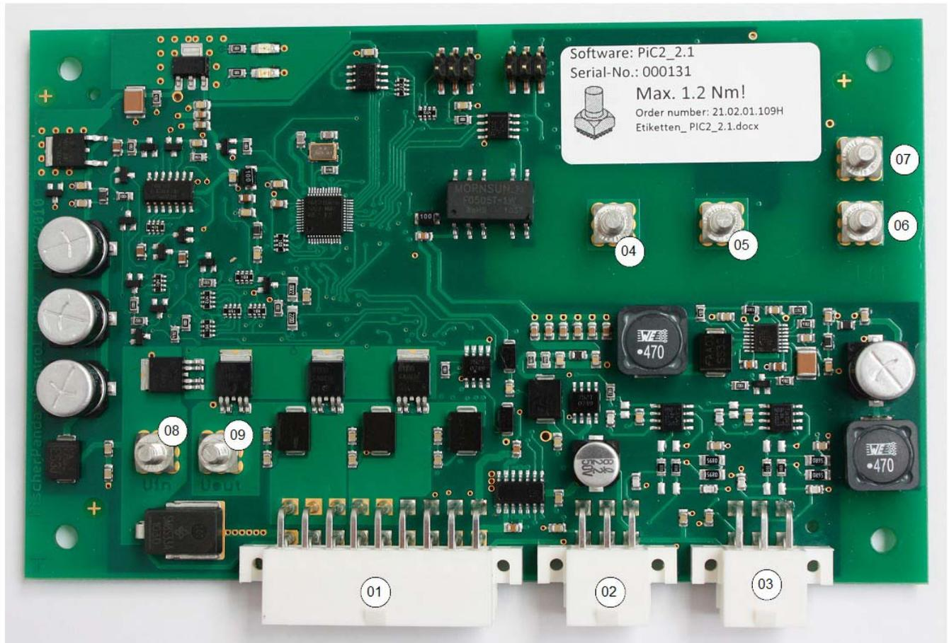
The Panda iControl2 controller is connected to the wire harness with the 18-pin jack. The centre 6-pin jack is designed for the Fischer Panda standard bus. The Panda iControl2 panel is connected to this jack. The Fischer Panda CAN bus is connected to the 6-pin jack at the bottom right of the circuit board. The configuration of the connectors is given in the subsequent tables. Siehe "Terminal assignments on the Panda iControl2 controller" auf Seite 156.
