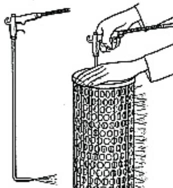
9. Check filter insert with penlight for damage.
