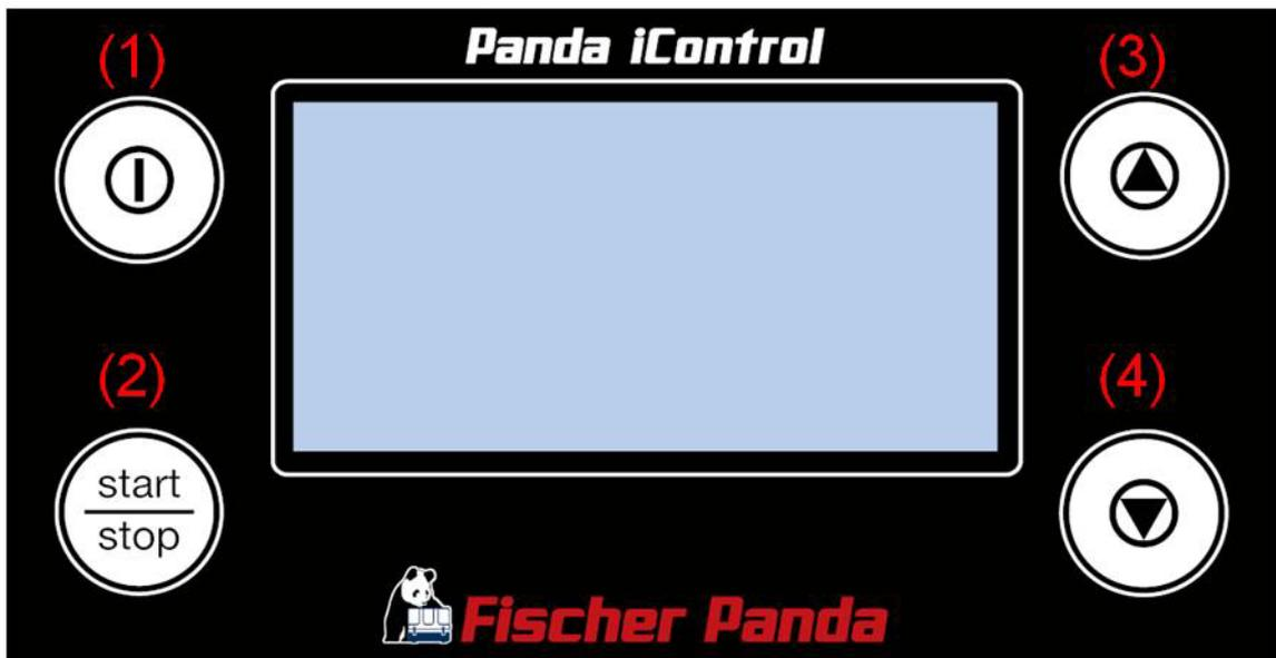
1. *On/Off button*: Switching the Panda iControl2 controller on and off
