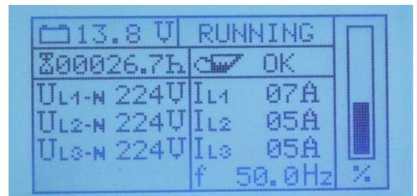
This screen provides the latest inverter phase voltages. You can access the inverter screen by actuating the cursor-up button while in operation mode.
