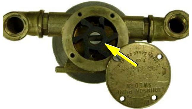
**Check to the impeller for damage and replace it if necessary.**
