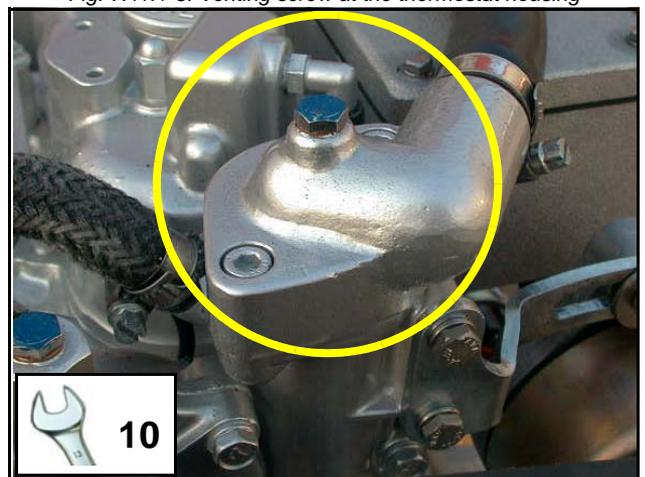
Fig. 7.11.1-3: Venting screw at the thermostat housing
