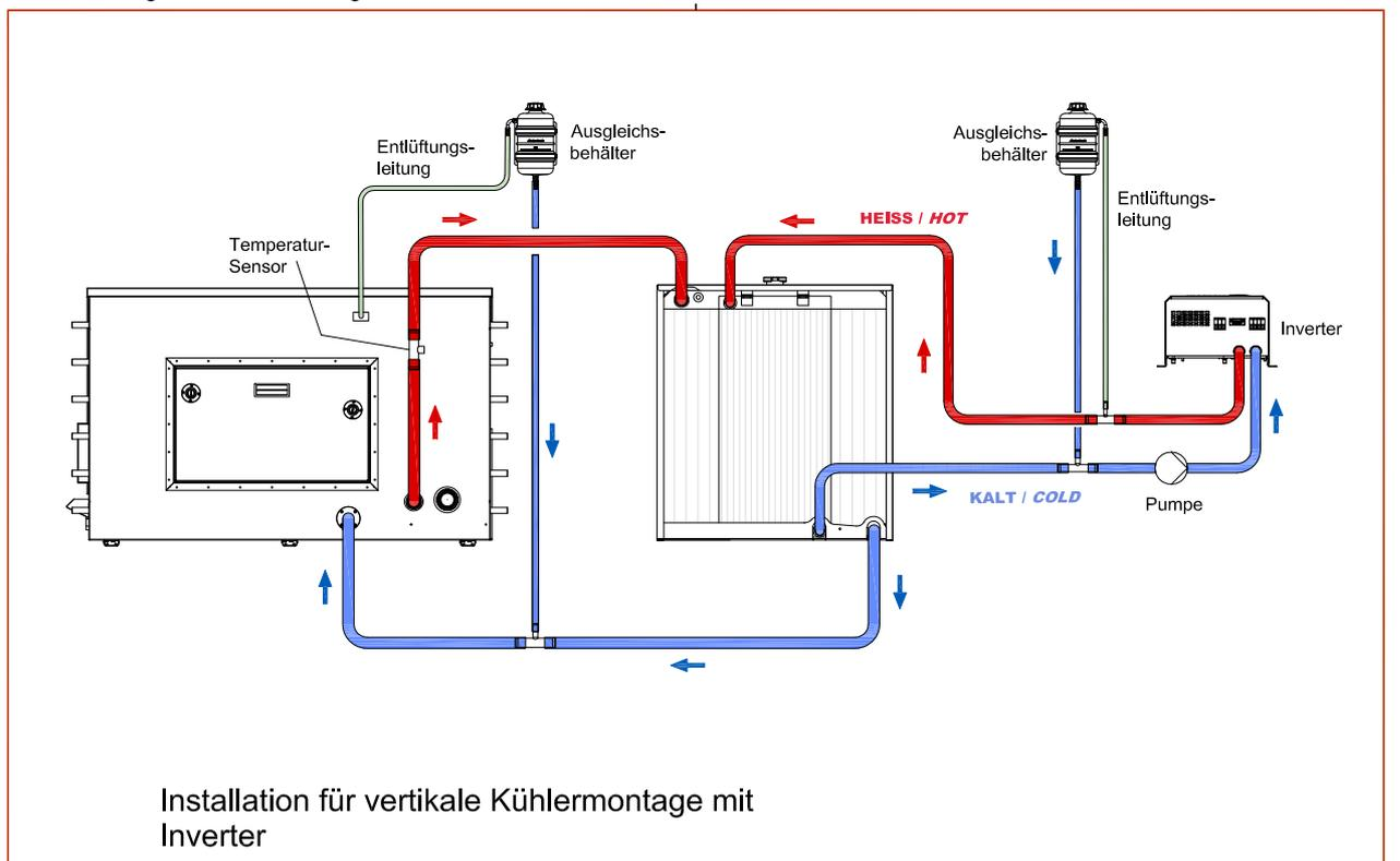
Fig. 10.10.1-2: Cooling water scheme if the Radiator is on the same level or lower than the Generator /Inverter
