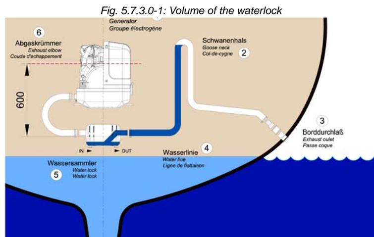
If there are any doubts, a verification can easily be made by temporarily using a clear-sighted hose (1) as exhaust hose. In that way, the cooling water level can be checked very easily.
