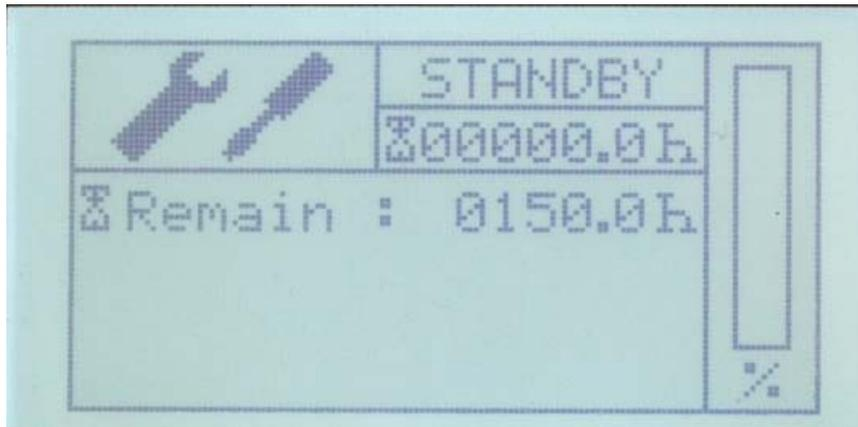
The total operating hours of the generator are given on the default display screen and on the service information screen. By actuating the cursor-up and cursor-down button in stand-by mode, the service screen can be accessed. This screen is marked with a screwdriver/spanner symbol. Here, the time until the next service is given. By actuating the cursor-up or cursor-down button, you can return to the default screen.
