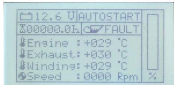
The autostart function will remain active even after the controller is switched off and on again with the On/Off button. To deactivate the autostart function, the flag in the EEPROM must be reset with "Disable" as described above.
