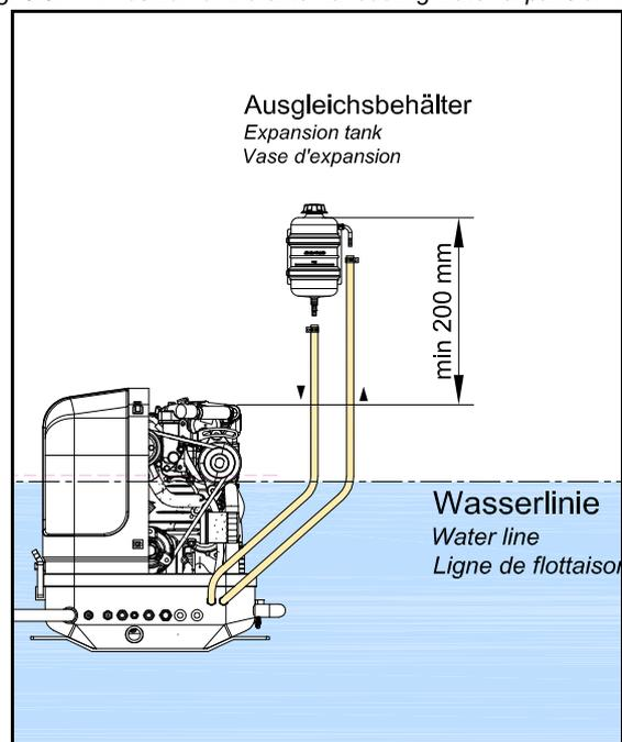
The external cooling water expansion tank may be filled only up to the lower edge of the lower tension tape (see note „max“) in the maximum filling level in cold condition.
