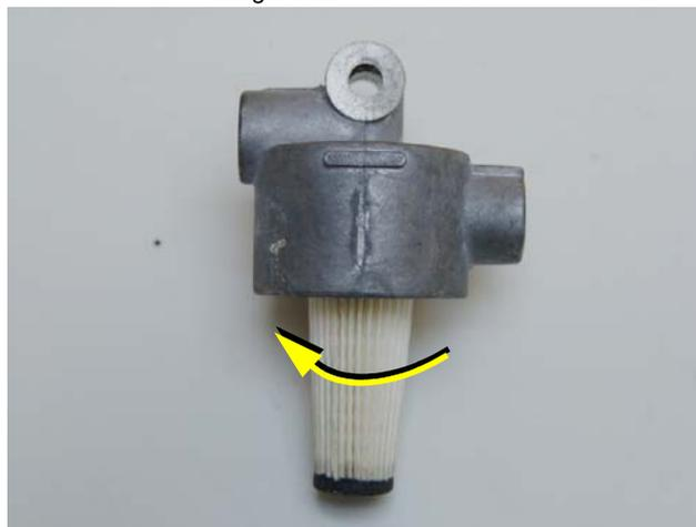
Screw the new filter element into the mount.
