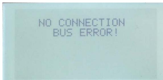
If the communication connection is lost, the generator shall be secured (open battery disconnect switches), and all plug-in connections and cables shall be checked for firm seating or damage.
