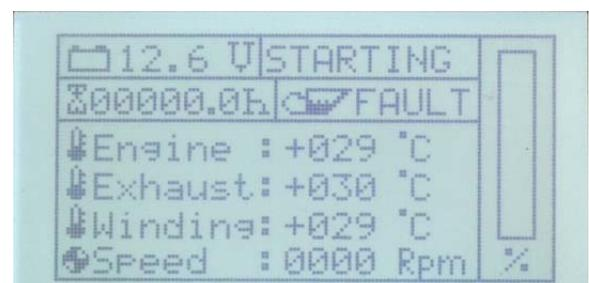
The controller will only perform one starting attempt. If the generator could not be started, the text output "STARTING FAILS" informs you of the failure of the generator starting attempt.
