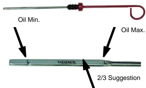
Oil should be refilled, if the oil-level is under 1/3 between the minimum and the maximum mark.
