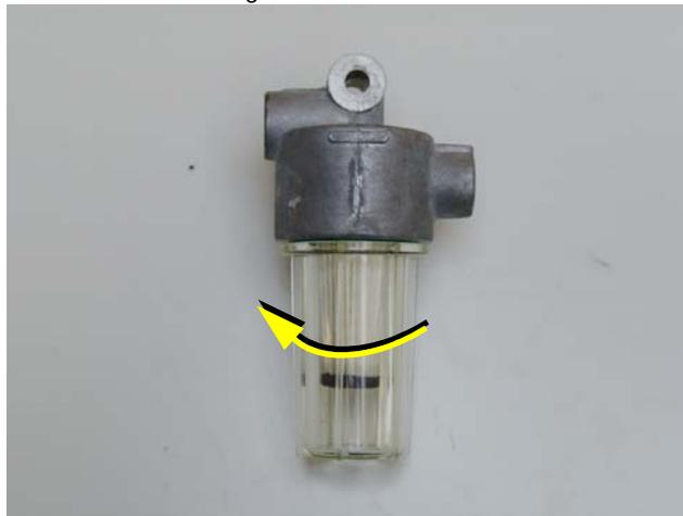
Unscrew the filter element from the mount (left hand rotation).
