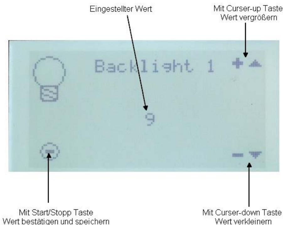
**In the sub-menus, set the desired values with the cursor buttons, and then confirm your settings with the Start/Stop button. Note:**
