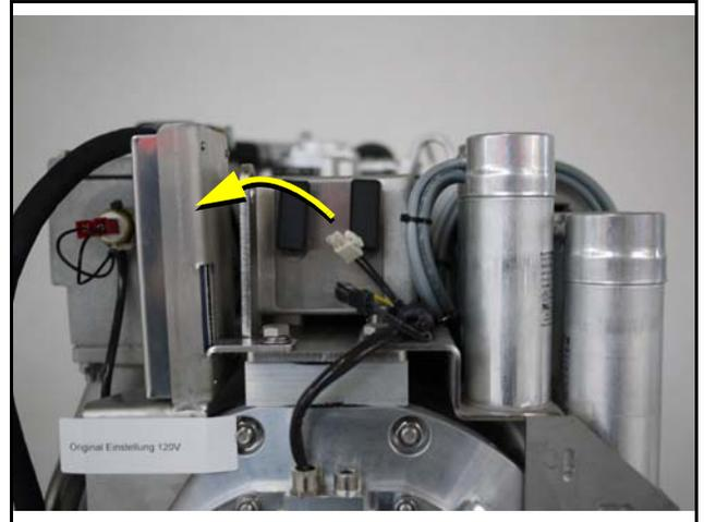
2. Tip the two fasteners 90°.
