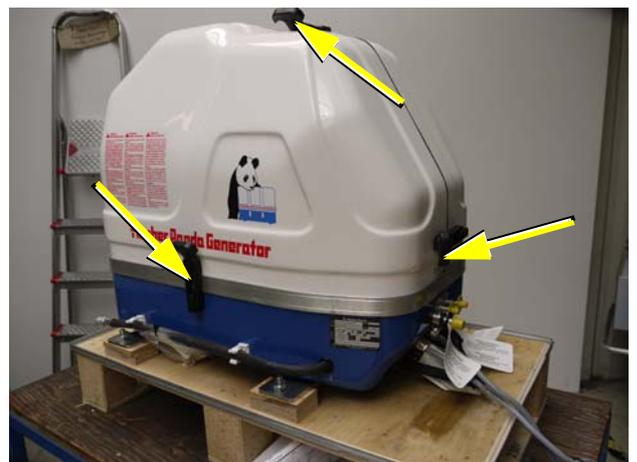
To open the lash closures pull the handle in arrow direction and lift the lash of the closure pin. After lifting off the lashes, the sound isolation cover upper part can be removed.
