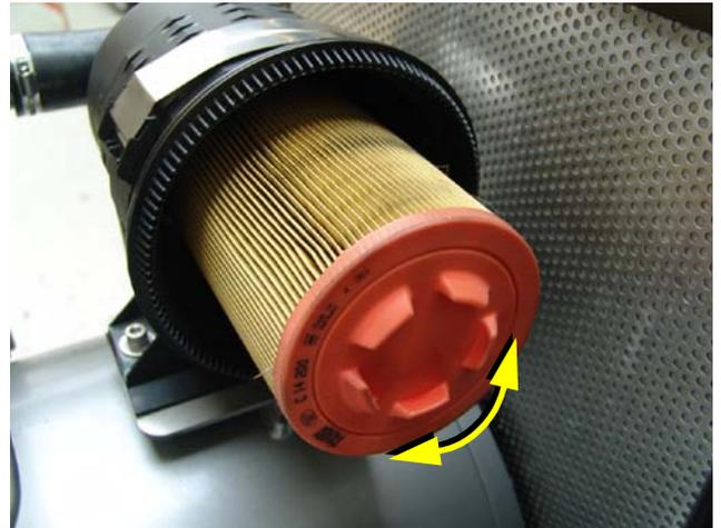
5. Clean the main element by blowing out with dry compressed air ( max. 5 bar) or replace the main element after 2 years at the latest.
