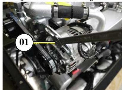
2. Loosen the fixing screw below the alternator.
