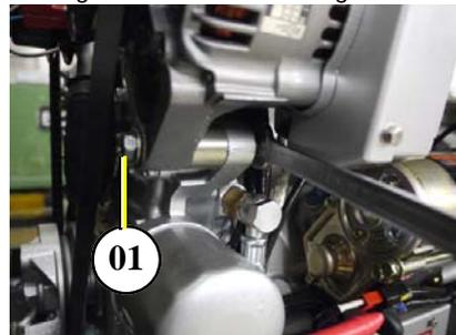
3. Push alternator towards the thermostat housing.
