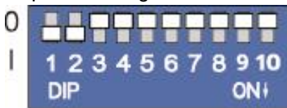
Figure 4: DIP switches (factory settings)
