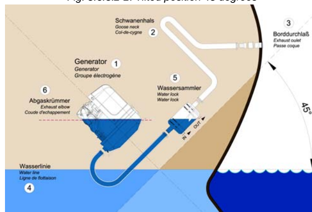
Fig. 5.6.3.2-2: Tilted position 45 degrees
