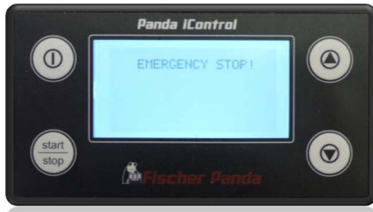
Fig. 12.5-2: Panel shows Emergency Stop
