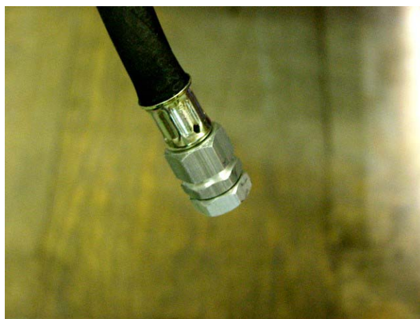
Fig. 7.7-2: Oil drain hose
