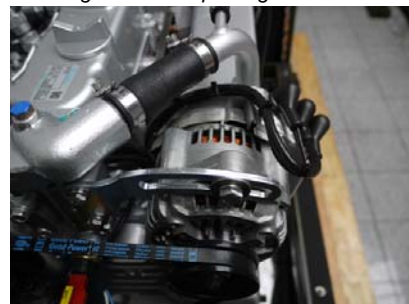
Fig. 7.11-3: Replacing the V-belt
