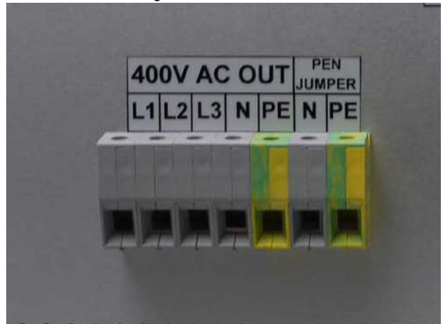
Fig. 10.5-3: PMGi AC out
