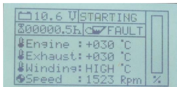
Fig. 15.1.1-2: Warning: „Winding temperature too high“
