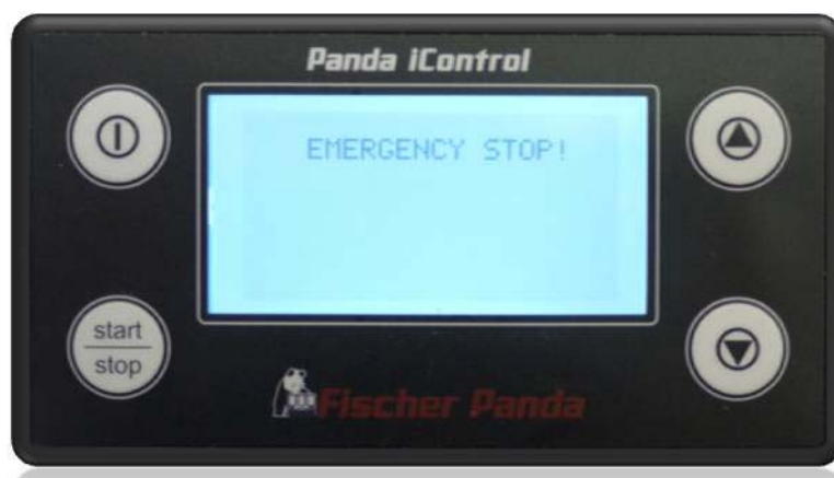
Fig. 13.5-2: Panel shows Emergency Stop
