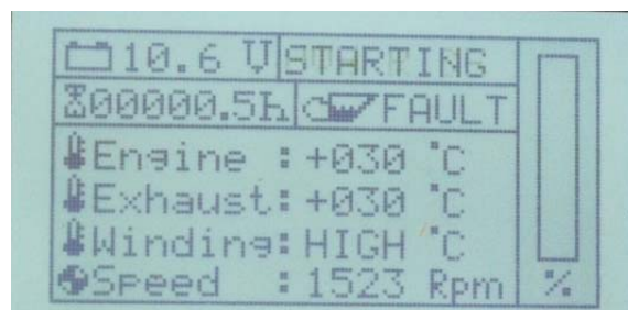
Fig. 16.1.1-2: Warning: „Winding temperature too high“
