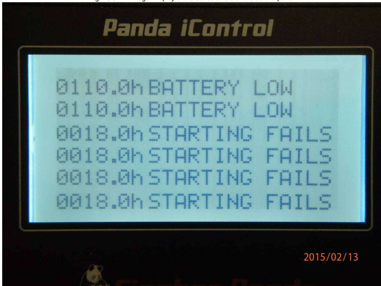
Fig. 16.3.7-1: Image: Display of the stored errors on the control panel
