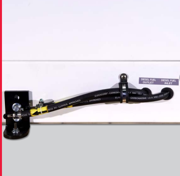
Fuel inlet and outlet
