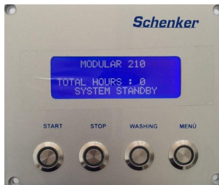
REMOTE CONTROL PANEL fig. 4-3
