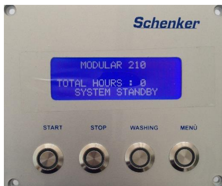
REMOTE CONTROL PANEL FIG. 4-3
