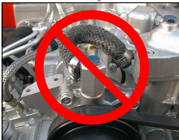
Fig. 9.10-5: Ventilation screw above the cooling water pump casing
