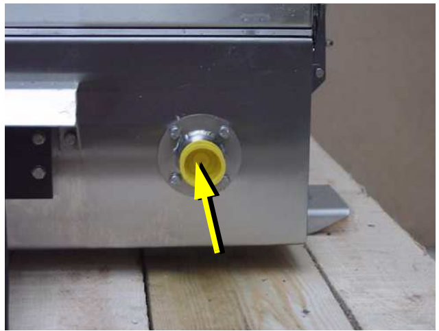
Fig. A.3.2-1: Raw water intake
