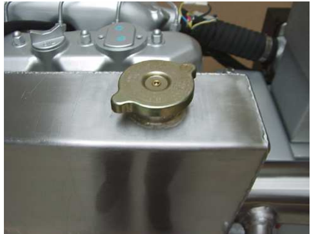
Fig. A.3.3-1: Cooling water filler neck
