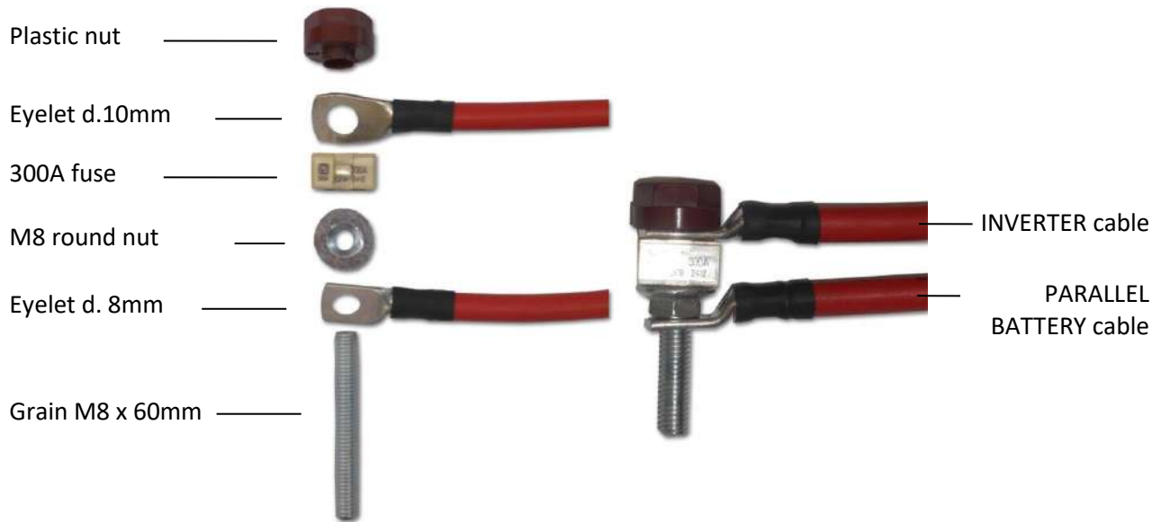
Pic.5 Protection Fuse
